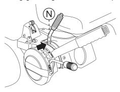
The lock button on the gear shift lever must be held in to engage reverse gear.
